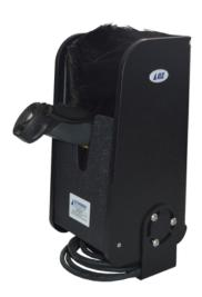
The *JLC Solutions* heated terminal holder eliminates the "Fogging" and "Freezing" on the laser scanner lens and on the terminal's display screen caused by temperature and humidity changes. This is accomplished by placing two thermostatically controlled heating pads designed to put the right amount of heat at both key points. This thermostatically controlled heated holder is a reliable solution on the issue of condensation with handheld terminals.
